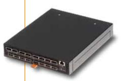
The innovative 16 port SAS 2.1 SAS Switch is a 1/2 wide, 1U high unit that has an optional rack mounting tray for dual switch requirements and support for Active SAS cables, which can extend the reach for two of the 24Gb/s ports (4 lanes each) to 20 meters. Embedded in the switch is a powerful management tool that enables full T-10 compliant zoning to individual SAS devices.
