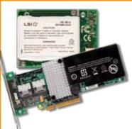
LSI offers a family of MegaRAID battery backup units (BBUs) and for use with our high-performance MegaRAID controller cards. The battery backup units protect the integrity of the cached data by providing power if there is a server failure or complete AC power failure.
