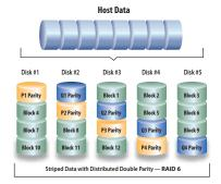
**RAID 6:** Two sets of parity data, P + Q, are striped across disks. RAID 6 safeguards against data loss during rebuild mode by allowing up to two consecutive drive failures for maximum fault tolerance.
